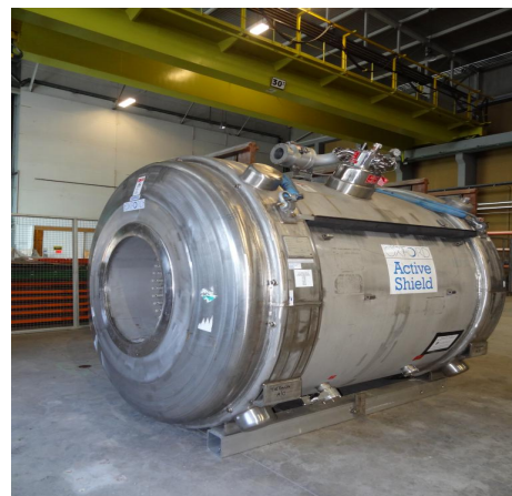
Figure 4: Helical Orbit Spectrometer, ex-MRI magnet delivered to CERN ISOLDE, April 2016
