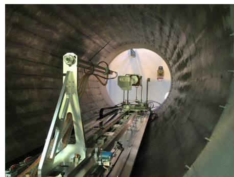
Figure 4a: Setting up detector and target systems inside the ISS magnet in preparation for in-beam tests at ISOLDE, CERN.
