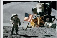
This is the bottom half of the lunar lander (called falcon for Apollo 15). The top part would later blast off the surface back into orbit around the Moon, but the bottom half was left behind.
