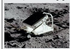
The LRRR is a bit like a giant bike reflector. When a laser is aimed at it from the Earth, it will bounce directly back. By timing how long this takes, scientists can work out the distance to the Moon!
