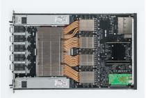
at FP16.16 and FP16.SR (stochastic rounding). The IPU-M2000 system has four IPUs, delivering approximately 1 PetaFlop of AI compute, and supporting ultra-low latency IPU-Fabric interconnect.
