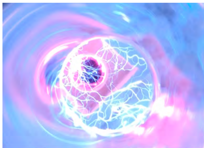
Photograph of the occurrence of arcing upon microwave irradiation of annealed graphene oxide based materials: This allows selective and ultra-rapid heating rates to be achieved leading to significant reduction in processing time.
