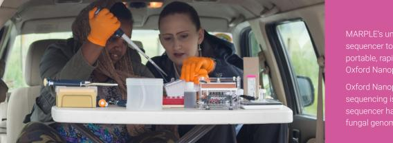
MARPLE's unique portability is thanks to the team's decision to use a minION nanopore sequencer to carry out their field pathogenomics technique. The minION sequencer is a portable, rapid DNA sequencer which plugs into a desktop computer. It was developed by Oxford Nanopore Technologies, a spinout company that benefitted from BBSRC investment.
