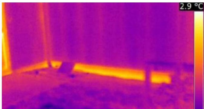
Image 1: Thermal image suggests there may be heat loss through the brick plinth at The Quarries.
