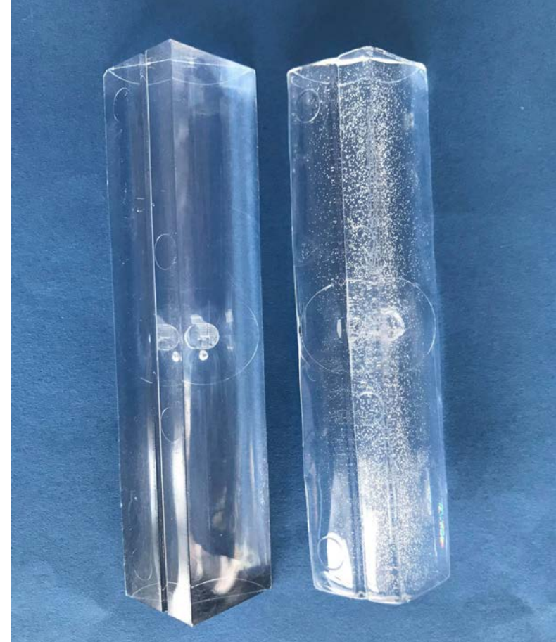
Room temperature vs 120 degree cycled polystyrene prism
