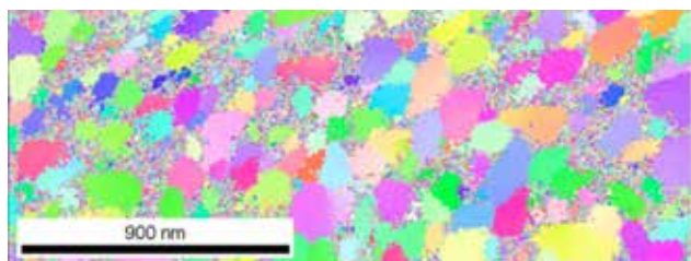
EBSD image showing grain sizes up to 250nm across at the surface of a film
