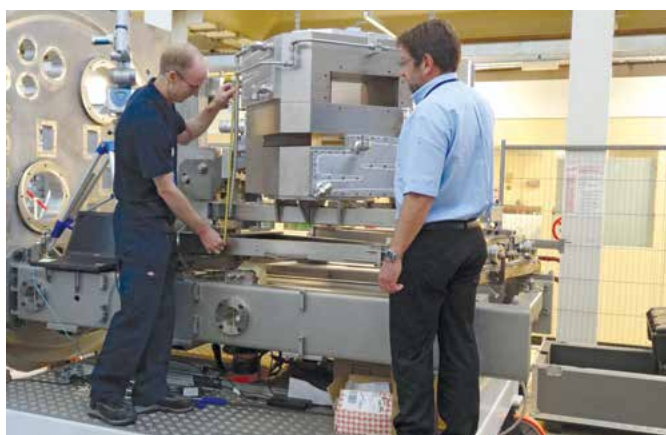
Andy Robinson and Graham Wallace assembling the MK II Beryllium Reflector onto the ISIS Second Target Station (TS2) test stand.
