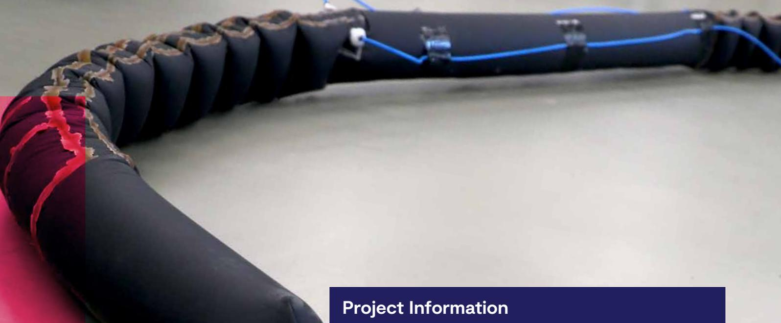
*The WormBot with multiple bends in 2D, similar to the potential underfloor use case*
