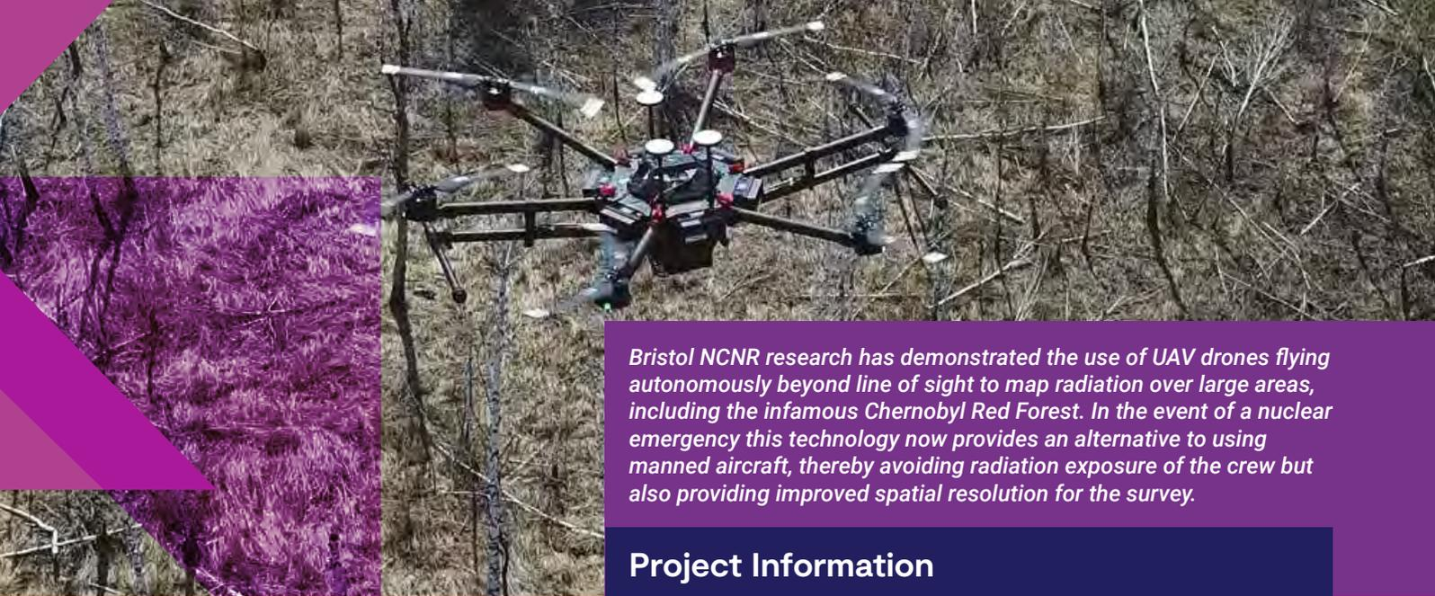
*Bristol NCNR research has demonstrated the use of UAV drones flying autonomously beyond line of sight to map radiation over large areas, including the infamous Chernobyl Red Forest. In the event of a nuclear emergency this technology now provides an alternative to using manned aircraft, thereby avoiding radiation exposure of the crew but also providing improved spatial resolution for the survey.*
