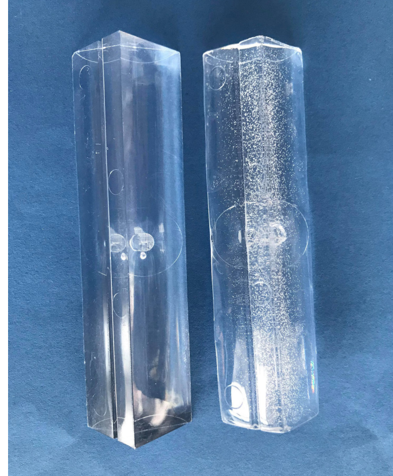
Prototype design for a 4-prism detector module coupled to KETEK SiPMs and transmitted via
