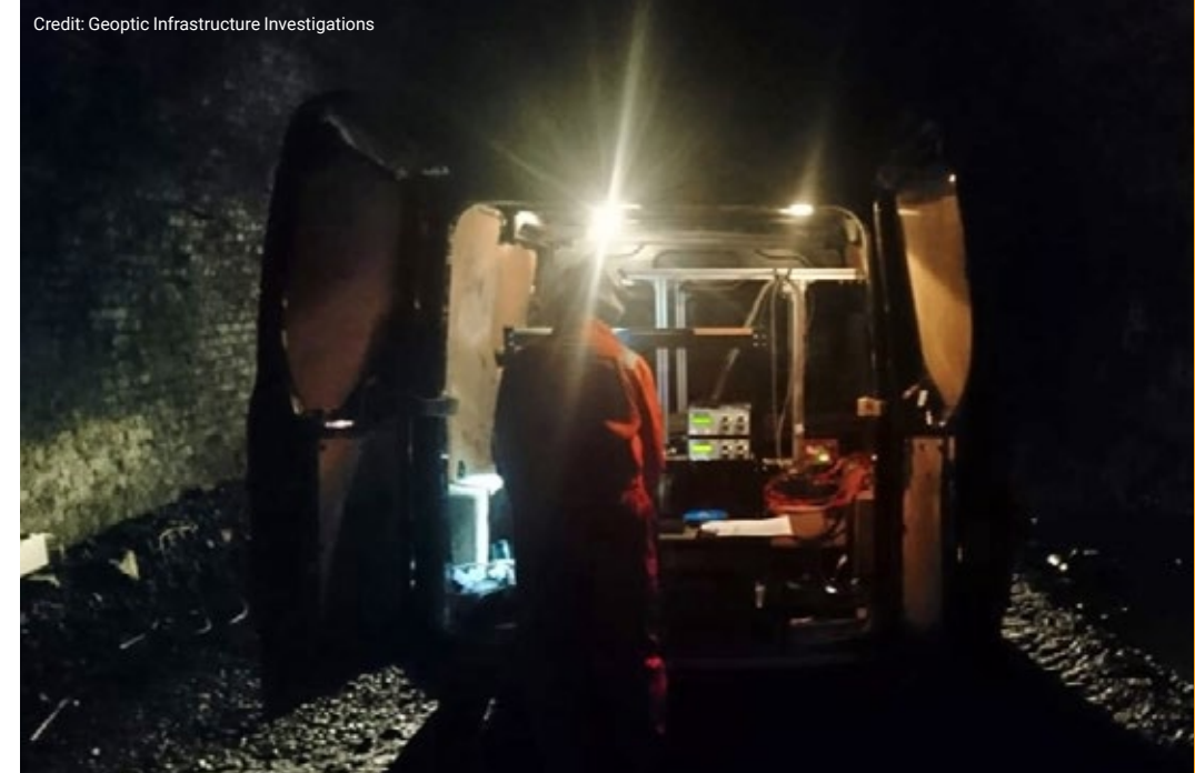
Muon tomography instrumentation imagining a railway tunnel
