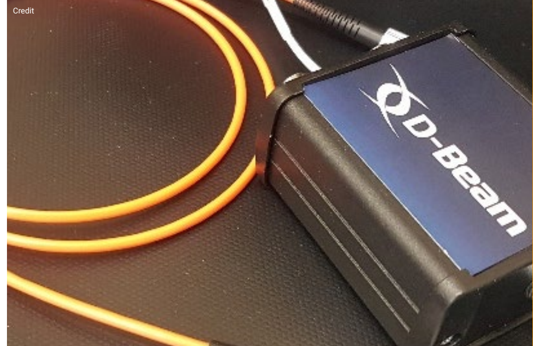
Optical beam loss monitor for accelerator optimisation. Image courtesy of D-Beam Ltd.
