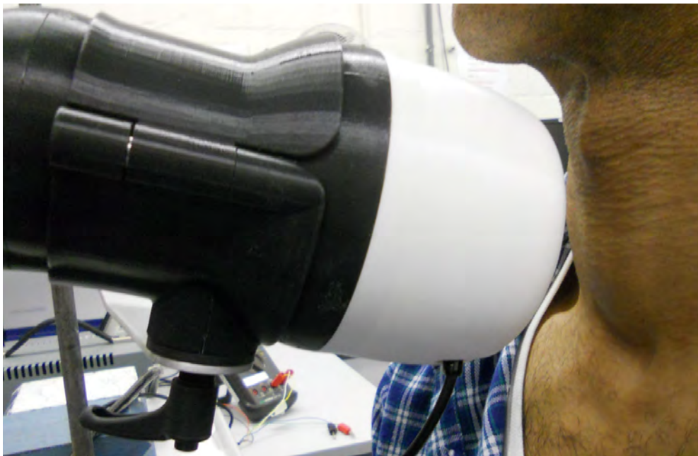
The hybrid gamma camera mounted on an articulated arm during clinical use.
