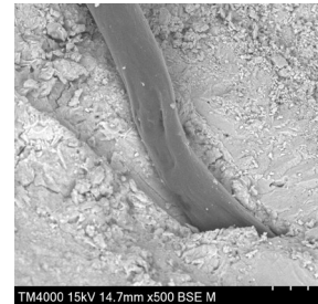
Micro-structural observations of plastic fibre integrated into the cementitious specimen
