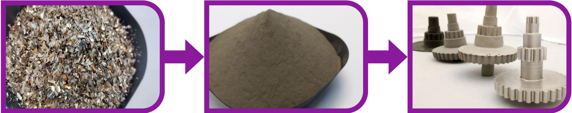
Scrap metal being turned into powder to create additively manufactured components
