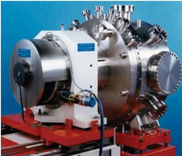
Figure 37, the first double-crystal monochromator manufactured by Vacuum Generators in May 1995 and delivered to the new Advanced Photon source (APS)
