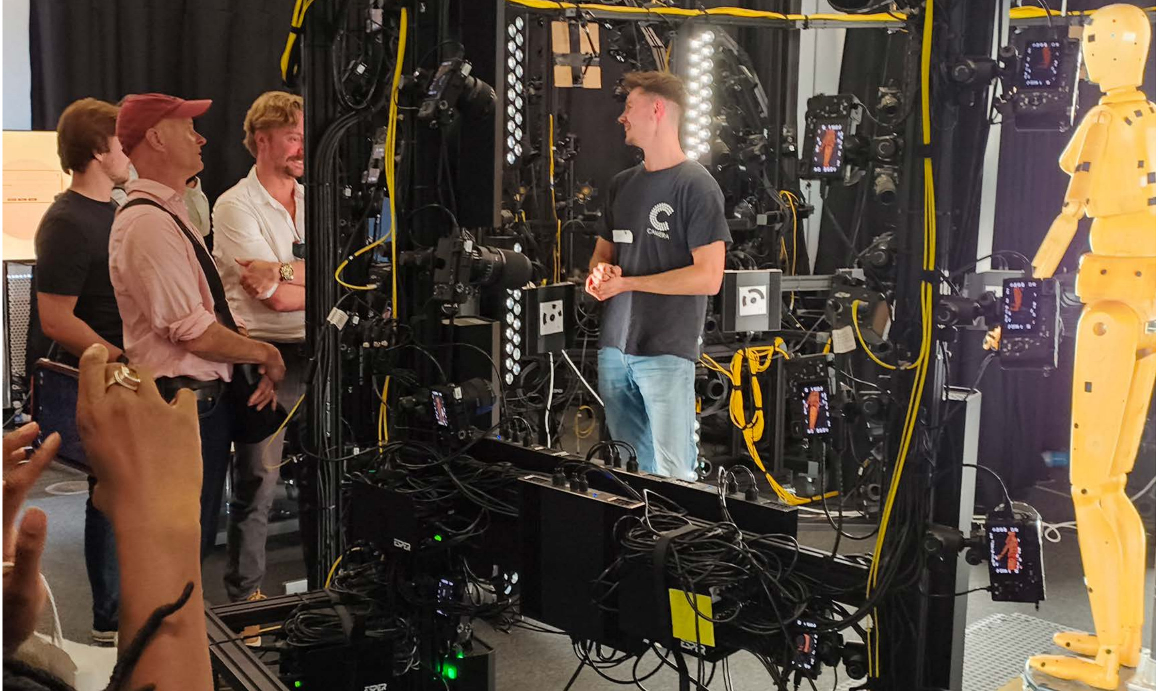
Full-body photogrammetry rig, CAMERA, Credit: Michelle Wu
